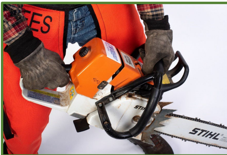
Figure 2.1.15—The correct way to hold a chain saw.
