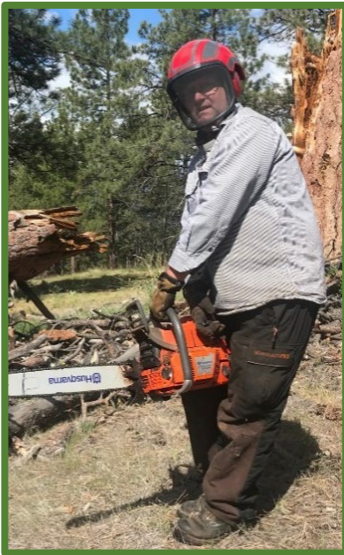
Figure 2.1.18—Starting a chain saw between the legs.
