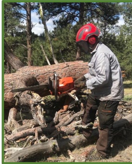
Figure 2.1.19—Starting a chain saw supported by a log.
