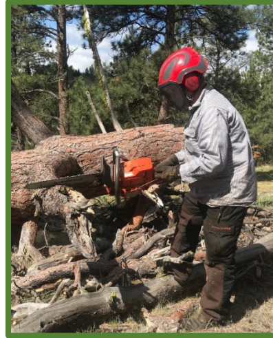
Figure 2.1.9—Starting a chain saw supported by a log.
